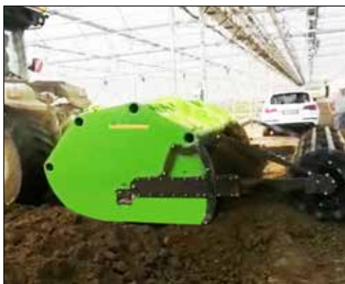
BIGROTAR brought (in a greenhouse) with a cage leveling roller automatic re-turn system
